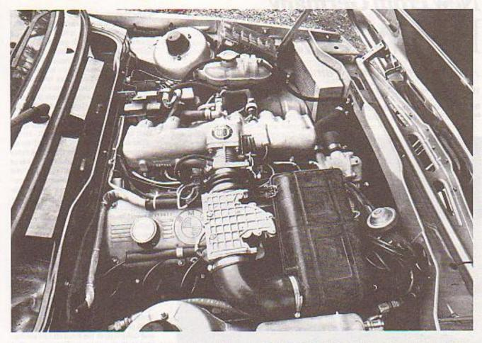
333i weighs 185 lb more than a production 320i tested in 1976. But the battery has been moved to the trunk which helps hold the increase on the nose to 2 percent. Weight distribution is a manageable 56/44 percent.
